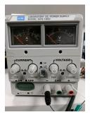
These power supplies are called **Bench(top) Power Supplies**. Most of the OPTIX modules you will encounter this semester or in ATEP will use a power supply because power supplies grant greater control over the voltage and current applied to a device than a battery. Locate the power supply in the OPTIX lab (it should be in the same cupboard as the blue box labeled 'Module 2', on the second shelf) and plug it into an outlet.
