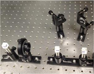
Place another polarizing beamsplitter cube directly behind the first one as shown in the figure. Carefully look at the orientation of the diagonal of the cube: You want the first cube to reflect the beam up, and the second cube to reflect the beam down, so
